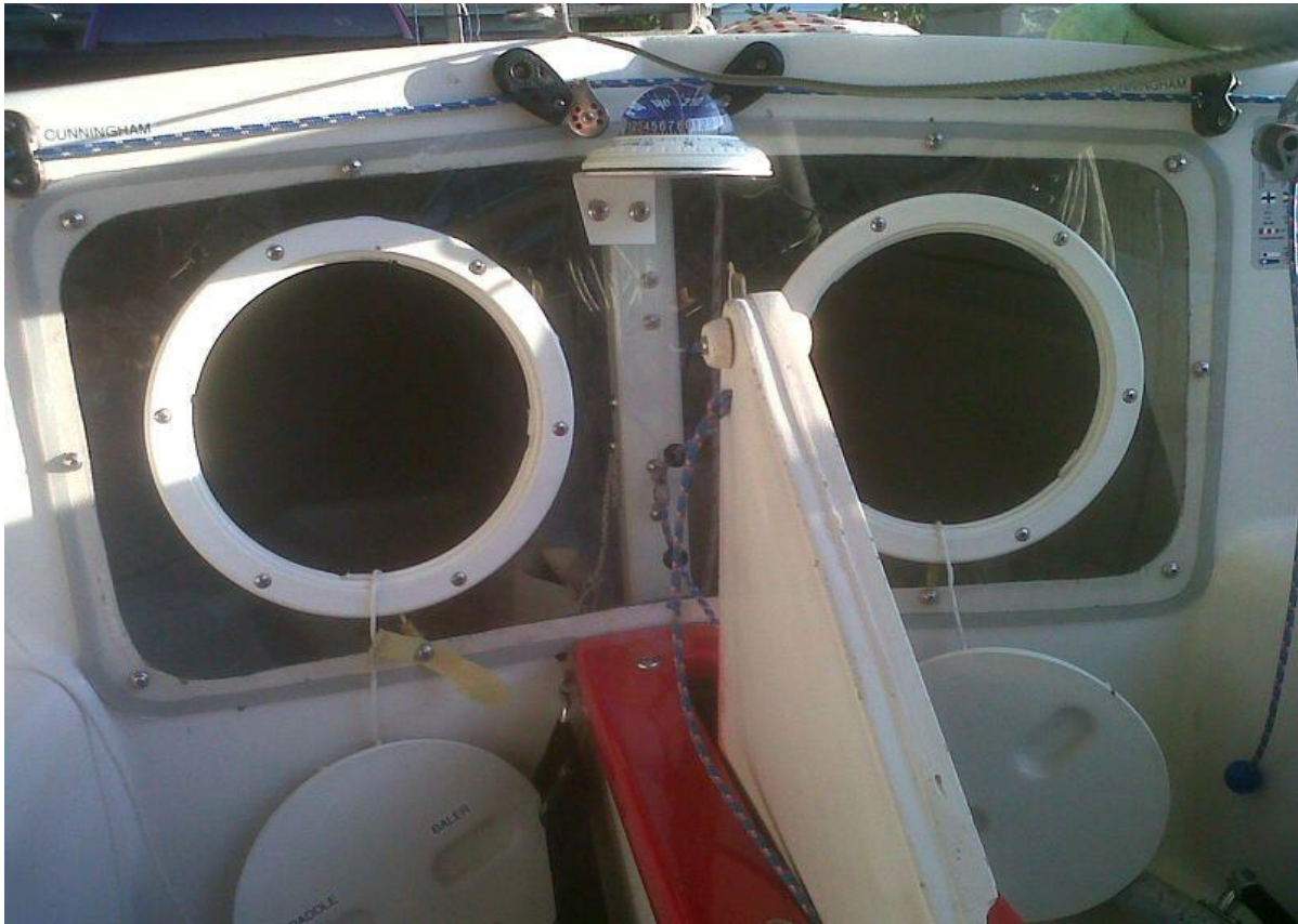
The finished cuddy cover in place.
