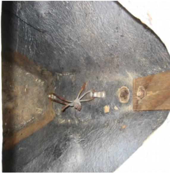
*Illustration 2: wire system attached to cutwater*
