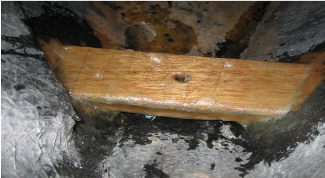
A 1/2" hole was drilled through both pieces. Through which a 1/2" stainless steel rod was inserted. There is a nut and washer above and below the boards. The bottom nut prevents the rod from being pulled upwards through the deck.
