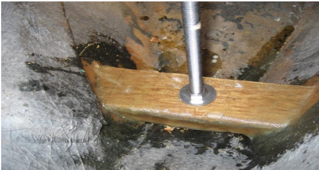
The top washer allows me to preload the deck by pushing from underneath with this washer that is pressed up towards the underside of the deck. I did this because I noticed that my spinnaker snout did
