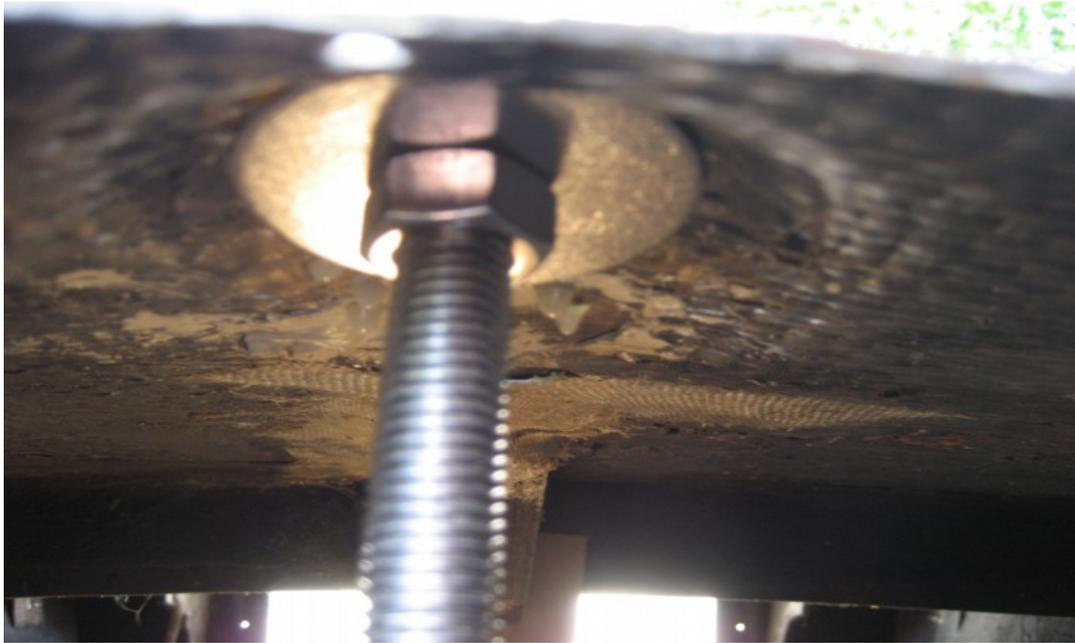
The 1/2" rod passes through the original furler hole. Between the washer underneath and the surface of the deck was filled with thickened epoxy. Yes, my epoxy skills are not the best, I plan to sand the whole deck at some point and repaint it, so it's ugly, but only for awhile.
