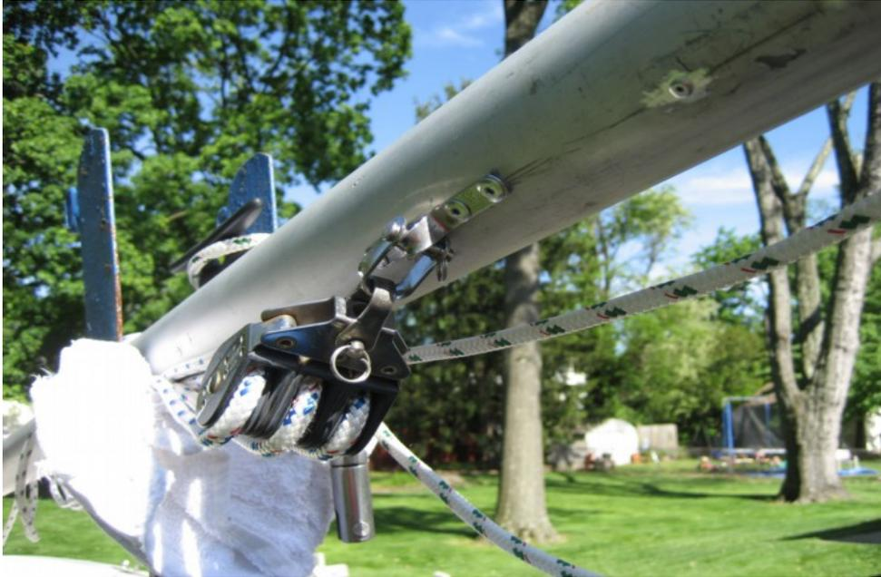
Once the mast is raised, I pull down on the triple block setup to tension the forestay. It rope is then tied off to a horn cleat attached to the mast. In hindsight I should have used a much smaller diameter block. The triple setup provides way more force tensioning the jib then is needed and the 38mm blocks seem to foul the jib a little when tacking. I plan to get smaller blocks and line.
