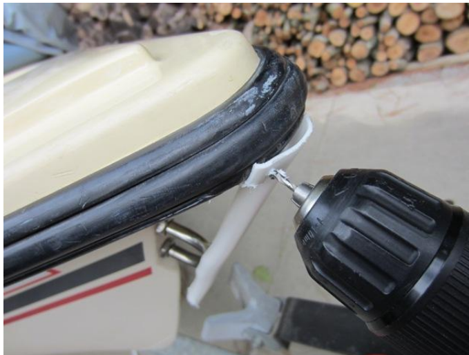
Drilling pilot holes.
